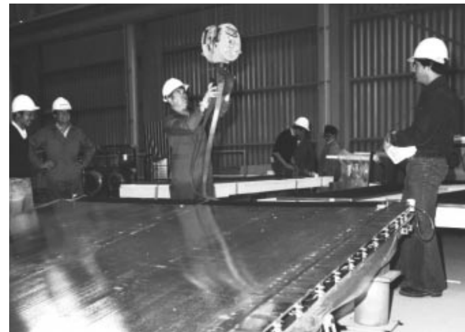
Figure 3. A Flash-Chamber Module Bobby Rechter (center) prepares to lift a flash-chamber module (silver plane.) Forty modules made up the neutrino detector for the E-225 experiment. At left are Minh Van Duong and Robert Burman; at the back are Peter Doe and K. C. Wang. The man at the right is unidentified.
